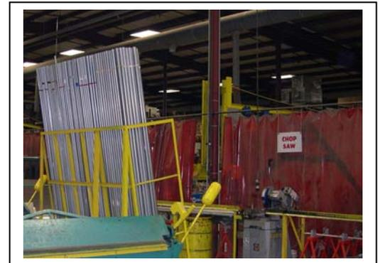
For the second work cell, the cold saw was moved to a central location. This, in turn, allowed the conduit rack to be in closer proximity to the saw. The rack used to be at the far end of the cutting bench so it took additional time to retrieve the conduit and cut it to length. Shifting the rack to the area directly behind the operator saves 20% off the time it took before the move.
