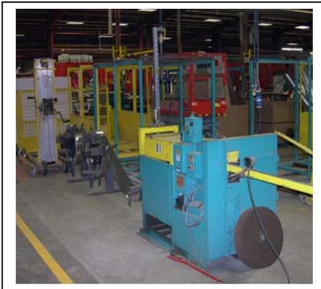
To create more floor space, two work cells and a portion of the shipping area were relocated. The first work cell involved moving the turning-vane machine closer to benches to cut down on the time tradesmen spend walking from one area of the shop to another. This move creates an ergonomic work area, eliminates unnecessary steps, and removes congestion in the fabrication area of the shop. This change helped save approximately 12 physical steps each time the machine is used.
